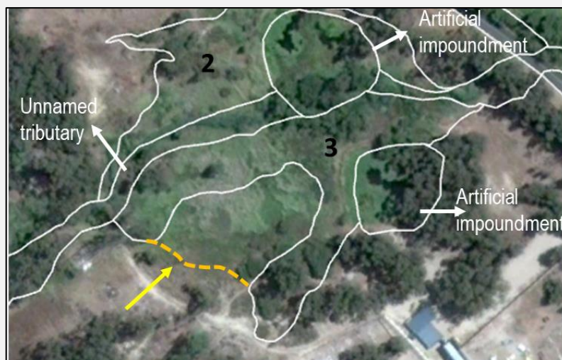
Figure 11: Digital satellite imagery (February 2014) of the area of unauthorised infilled material south east of Old Sir Lowry's Pass Road. No infilling is present in the wetland (yellow arrow) and the CVB wetland is continuous in this area. Orange dotted lines depict where the wetland edge was previously based on digital signatures. Numbers depict the different CVB wetlands.
