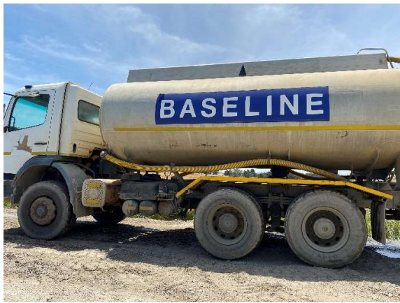
Water tanker available for dust suppression along the route.
