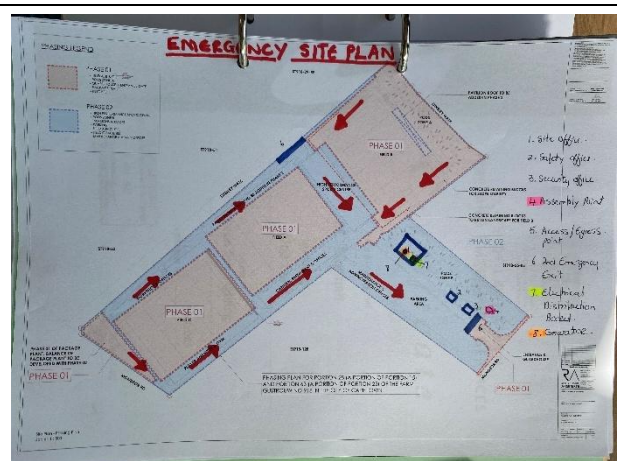
Emergency Assembly and Exit Points.
