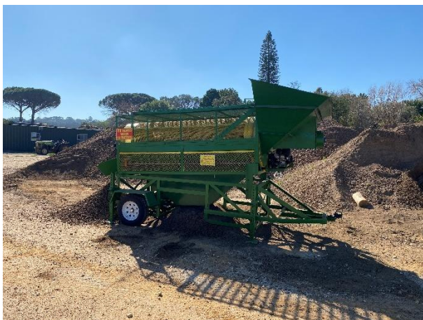
Vibrating screen used for the separation of rocks by size.
