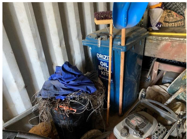
Oil spill kit available on-site within a lockable container.
