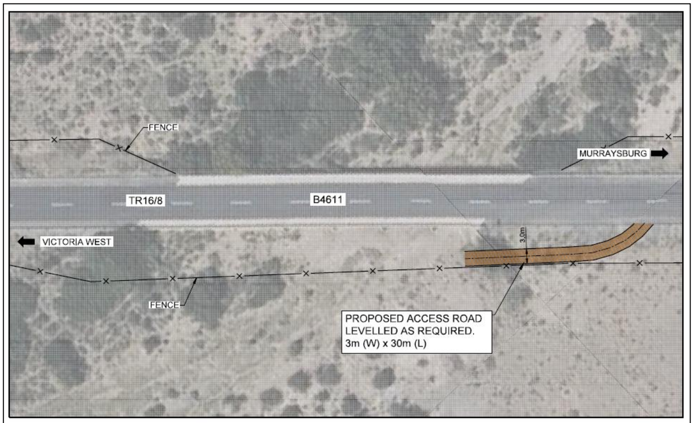
Figure 1: Proposed bridge access at B4611.
