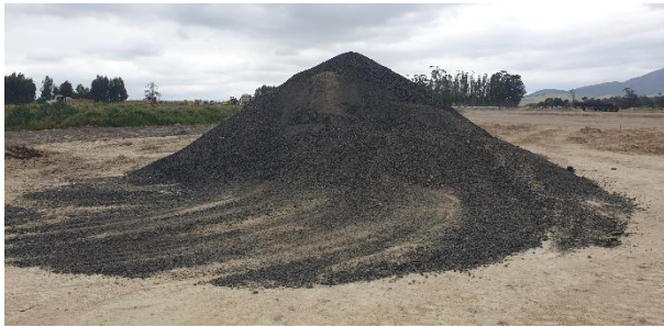
Crushed stone aggregate prepared for asphalt surfacing.
