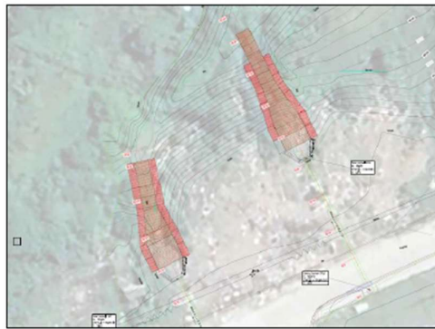
Figure 10: Plan view of stepped gabion hydraulic structures terminating at a non-perennial stream of the Meul River (Site 69).
