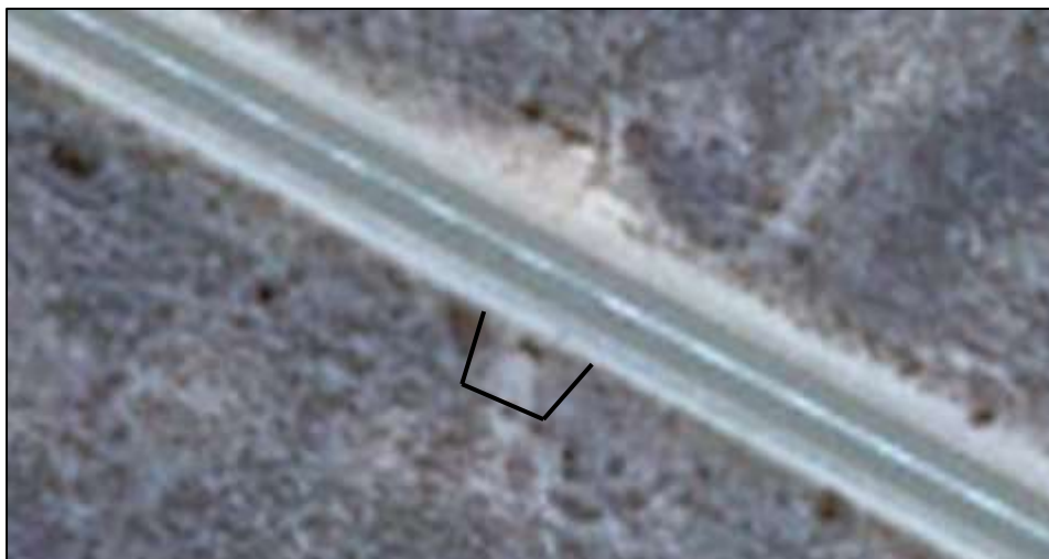
Figure 13: Demarcation example for areas with little to no embankment slope
