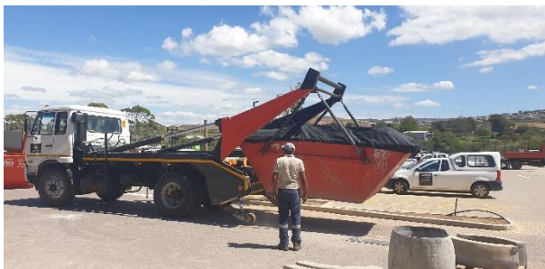
Waste removal truck collecting skips from the construction site.
